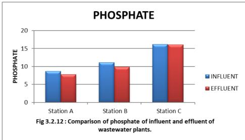
Phosphate is one of the contributing factors in the increased eutrophication of lakes and natural water bodies. Here, there is a decrease in phosphate concentration by the three industries. Station A decreased the phosphate concentration by 8.39%, station B by 10.17% and station C by 0.30%. i.e. station B is more efficient among the three.
