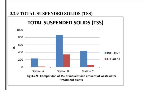
Total suspended solids play an important role in waste water treatment. TSS test results are routinely used to assess the performance of conventional treatment processes. In present study, the TSS in the Influent of the treatment Plant is between 234.1mg/L to 860.4 mg/L. And a considerable decrease in all the samples after treatment.
