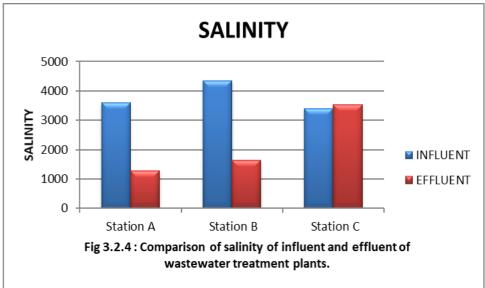
Salinity is the total concentration of the dissolved salts in water. Conductivity and salinity have a strong correlation. Salinity is important as it affects the dissolved oxygen solubility. The higher the salinity, the lower the DO concentration. In case of station A and station B, salinity is decreased from 3604mg/L to 1288.8mg/L and 4352mg/L to 1650mg/L respectively. But in case of station C, shows a slight increase in salinity in the effluent.
