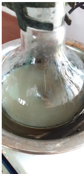
Hibiscus petal extract + Zn sulphate + sodium hydroxide after 2 hours of stirring
