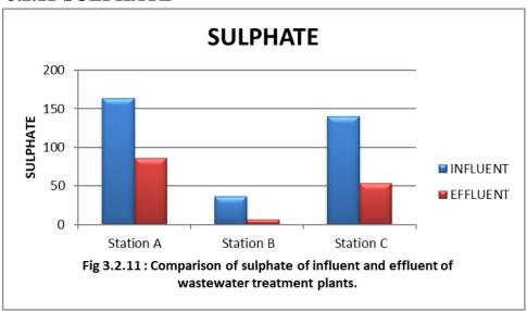
Most of the seafood industrial effluents contain a high concentration of sulfate. Anaerobic treatment is widely used for the treatment of high organic content wastewater. Here the sulfate concentration is reduced after the treatment process of all the three industries. Station A decreased the sulfate concentration by 47.65%, station B by 82.48% and station C by 61.54%. i.e. station B is more efficient among the three.
