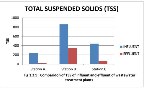
Total suspended solids play an important role in waste water treatment. TSS test results are routinely used to assess the performance of conventional treatment processes. In present study, the TSS in the Influent of the treatment Plant is between 234.1mg/L to 860.4 mg/L. And a considerable decrease in all the samples after treatment.
