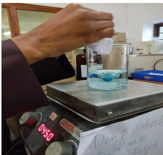
PEG is dissolved and copper acetate is monohydrate is added
