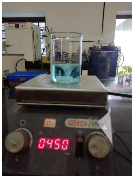
Magnetically stirred at 450RPM
