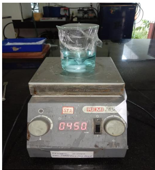
The beaker is closed and stirred for 24 h
