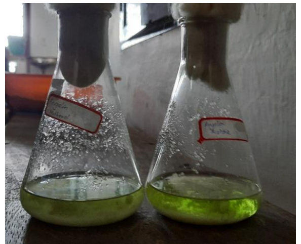
Figure 2 : Fruit pulp soaked in methanol and acetone
