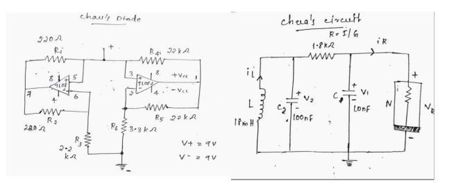
Alongside the Chua diode, the circuit comprises two capacitors and three operational amplifiers interconnected in a specific configuration.
