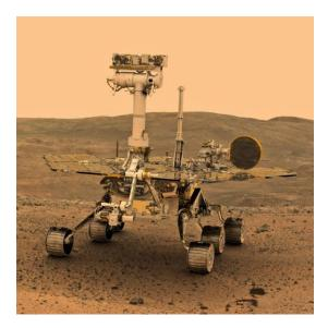
The Opportunity rover was a robot vehicle that explored Mars from January 2004 to June 2018 as part of NASA's Mars Exploration Rover mission. The mission aimed to investigate the planet's surface and geology to uncover any evidence of past water on Mars and to look for indications of ancient or current life.
