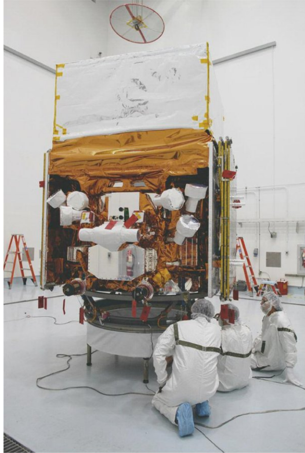
Figure 5.1: 1 The Fermi Gamma-Ray Space Telescope being prepared for launch vehicle integration at Cape Canaveral. On top is the LAT with its reflective covering. Six of the GBM NaI detectors and one BGO detector can be seen on the side of the spacecraft. Photo credit: NASA/Kim Shiflett(Meegan et al. 2009).
