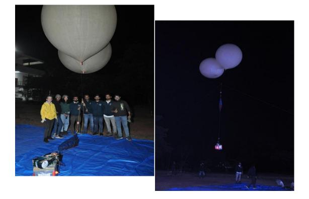
High altitude balloon launches is a type of experimental technology used for research and educational purposes. The main objective of these launches is to send scientific payloads, such as cameras, sensors, and other equipment, to the upper reaches of the atmosphere for data collection and analysis. The balloon itself is typically filled with helium or hydrogen, which allows it to reach altitudes of 100,000 feet
