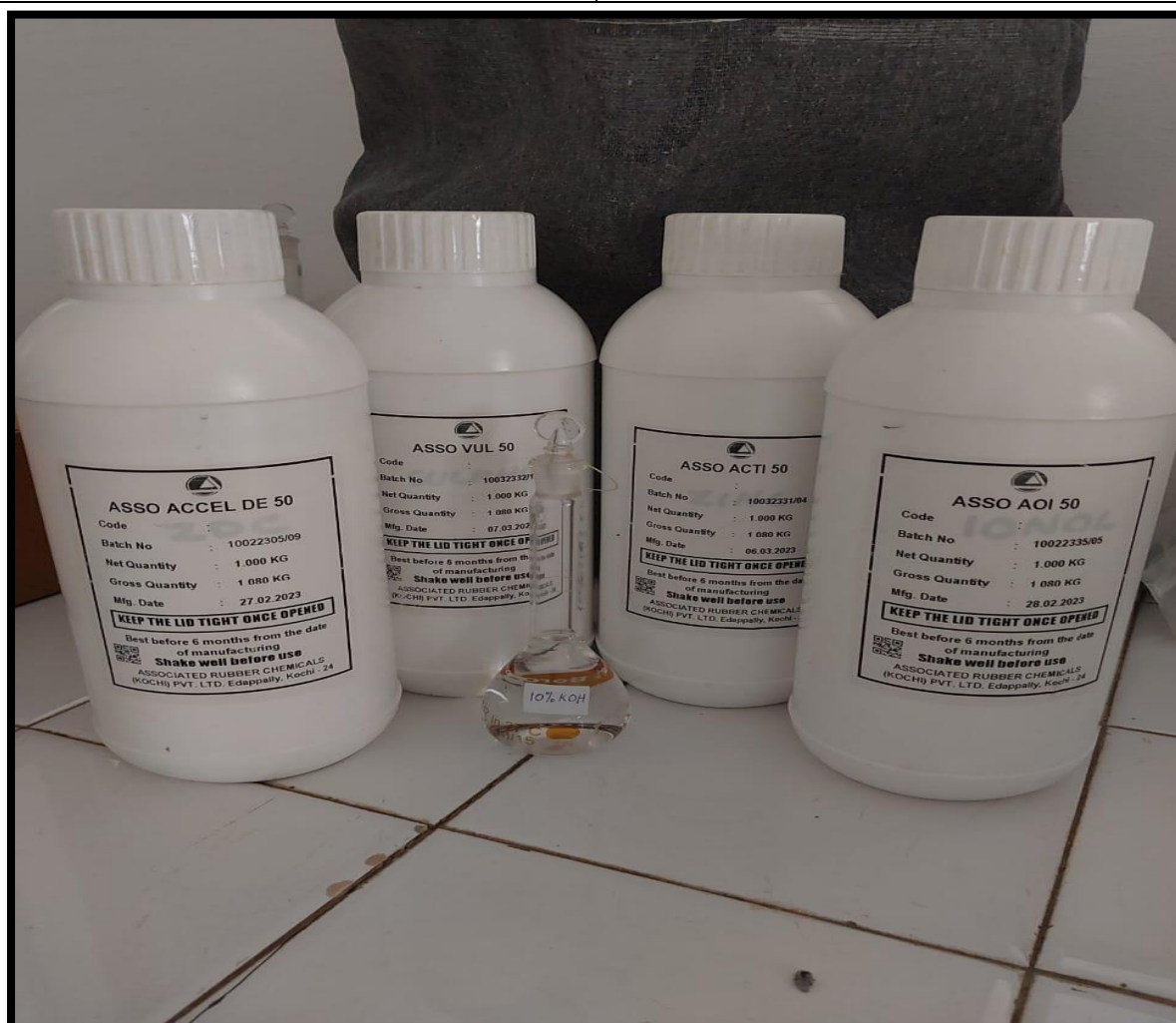
Fig 3.5 Chemicals used for compounding ( accelerator, vulcanizing agent, activator, antioxidant, KOH )
