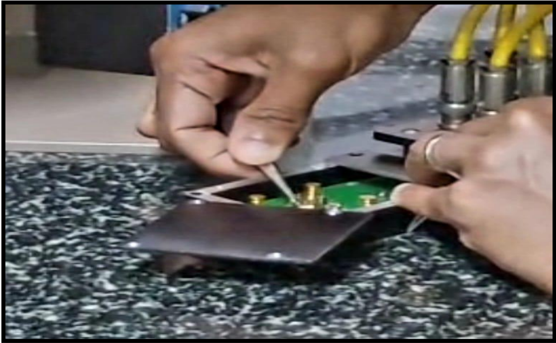
Fig 3.10(a) Four – probe of van der Pauw apparatus
