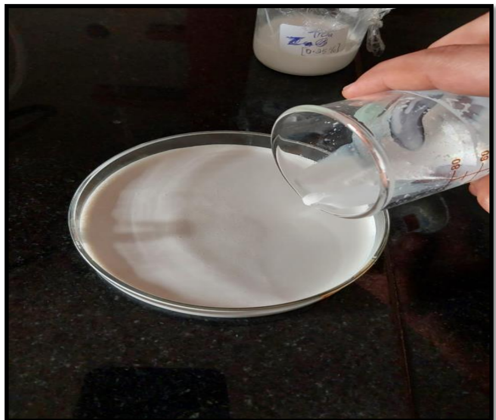
Fig 3.7 After stirring the mixture is transformed in to petri dish
