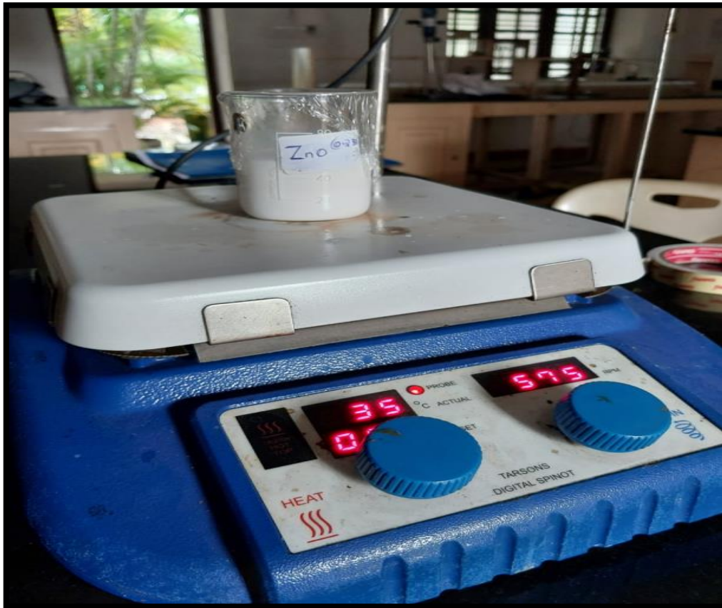
Fig 3.6 Natural rubber along with compounding chemicals and nanofillers (here ZnO) is kept on magnetic stirrer
