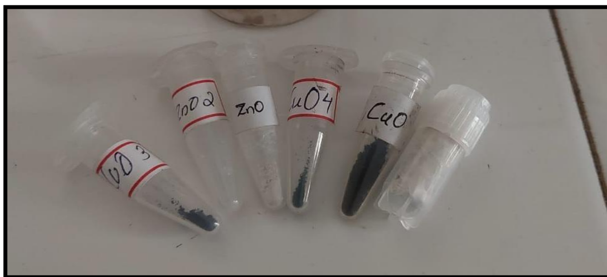
Fig 3.3 Synthesized CuO, ZnO and TiO 2 nanoparticles
