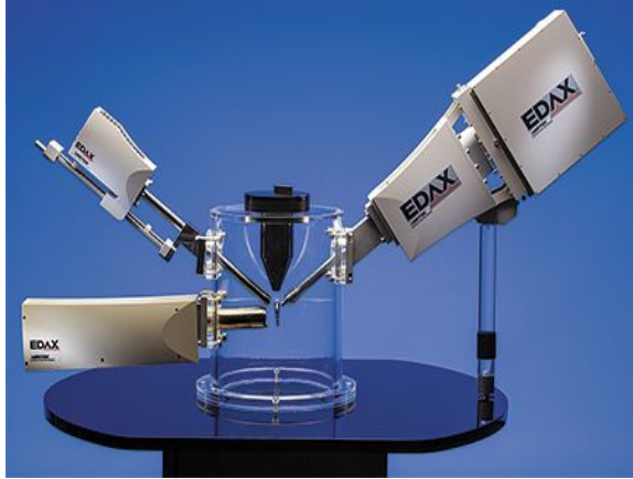
Figure 2.7 : Energy-dispersive X-ray analysis (EDAX).
