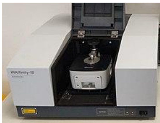
An example of an FTIR spectrometer with an attenuated total reflectance (ATR) attachment
