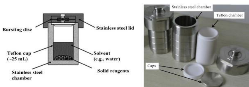
Parts of Teflon Autoclave used for Hydrothermal Method
