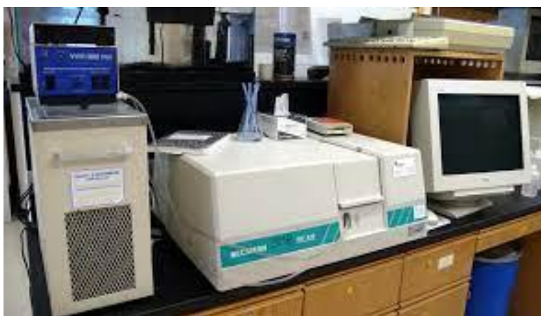
Beckman DU640 UV-Vis spectrophotometer:-
