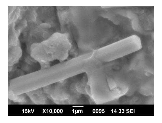
The microstructure of the silver nanoparticles is observed from SEM images. The silver nanorods are clearly seen in the image.
