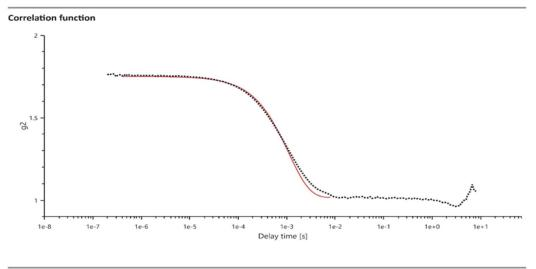
The particle size is found to be 715.6 nm which is actually the size of the solvated nanoparticle.
